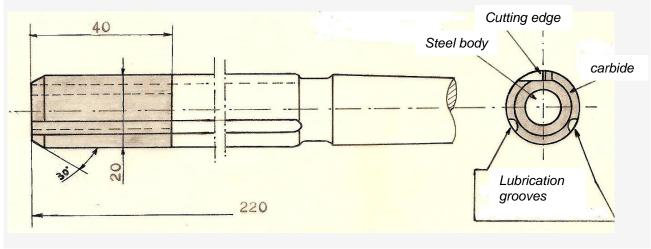
Figure N°8- Single cutting edge reamer
