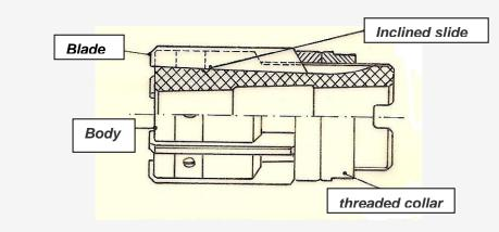
Figure N°5- Adjustable blade reamers sleeve type
