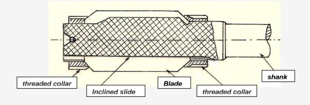
Figure N°4- Adjustable blade reamers shank type
