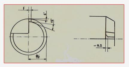
Figure N°7 - Rake angles of a single cutting edge reamer
